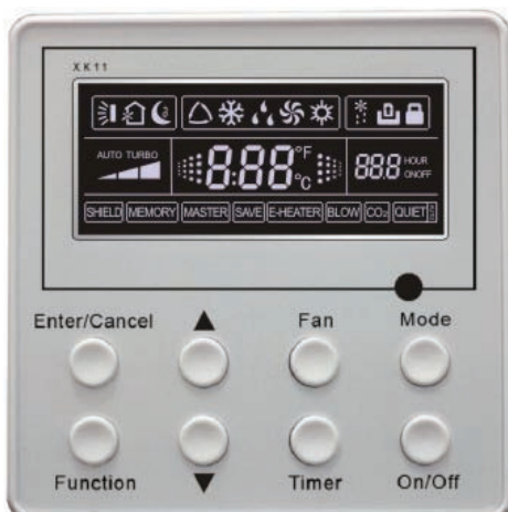
Fig.3.1 Outline of wired controller
