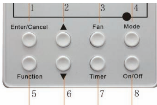
Fig. 3.3Silk screen of buttons
